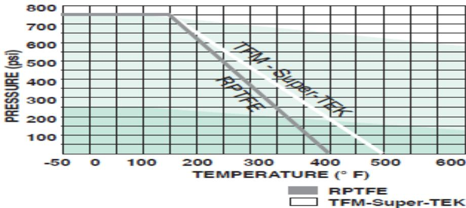
Rating Curve applies to both "L" and "T" port configurations. All Values conform to ANSI Class pressure ratings. They are rated for a maximum differential pressure of 275 psi, and a maximum temperature of up to 550 °F. WCB - 285 psi Max. Complies with ANSI B16.5 and B16.34 standards.
